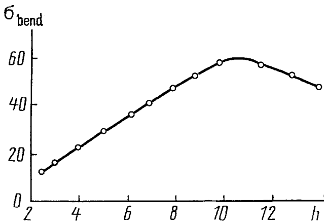
Fig. 2. Plot of the ultimate bending strength versus the plate thickness h (T. A. Ketegenov and A. N. Karabalin's data). \sigma_{bend} , MPa; h , mm.
